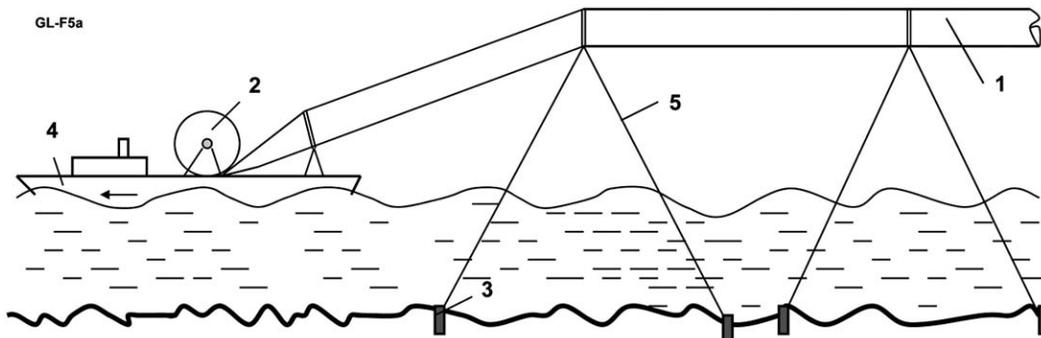
Fig. (5). Building the offered gas pipeline by sea ship. Notation (1) Gas pipeline (2) Roll from the inflatable film tube (3) Load for fixing tube to sea bottom (4) Support ship (5) Tensile links.
