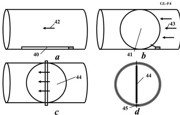
Fig. (4). Gas valve. (a)-(b) Inflatable valve, (c)-(d) Flat valve. Notations: 40 - inflatable valve in compact position, 41 - inflatable valve in fill out position, 42 - gas flow, 43 - gas pressure, 44 - flat choker disc.
