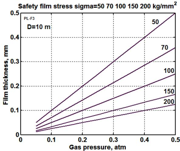
Fig. (9). Film thickness via gas pressure and the safety film stress for the tube diameter  $D = 10 \text{ m}$ .
