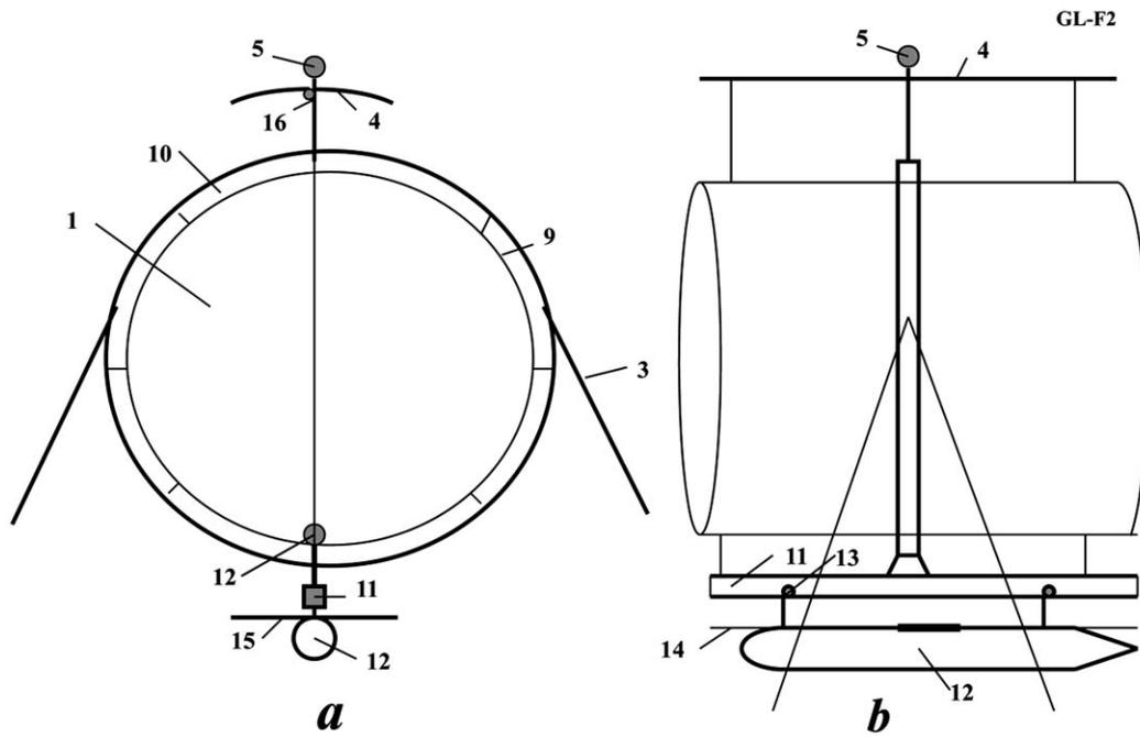
**Fig. (2).** Cross-section and support ring of aerial pipeline. (a-left) front view, (b-right) side view. Notations: 9 - double casing, 10 - rigid ring, 11 - monorail, 12 - wing load container, 13 - rollers of a load container, 14 - thrust cable of container, 15 - container wing. Other notations are same as in Fig. (1).
