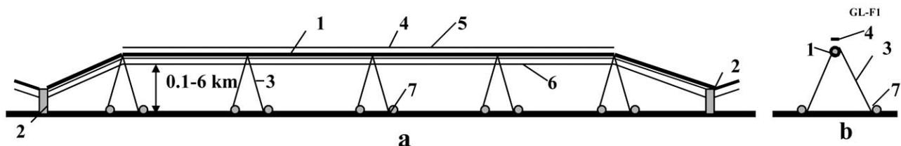
Fig. (1). General view of air pipeline between two compression (pump) stations. (a, left) Side view, (b-right) front view. Notations: 1 - pipeline in atmosphere, 2 - compression station, 3 - tensile stress element, 4 - support wing device, 5 - aircraft warning light, 6 - load (container) monorail, 7 - winch.
