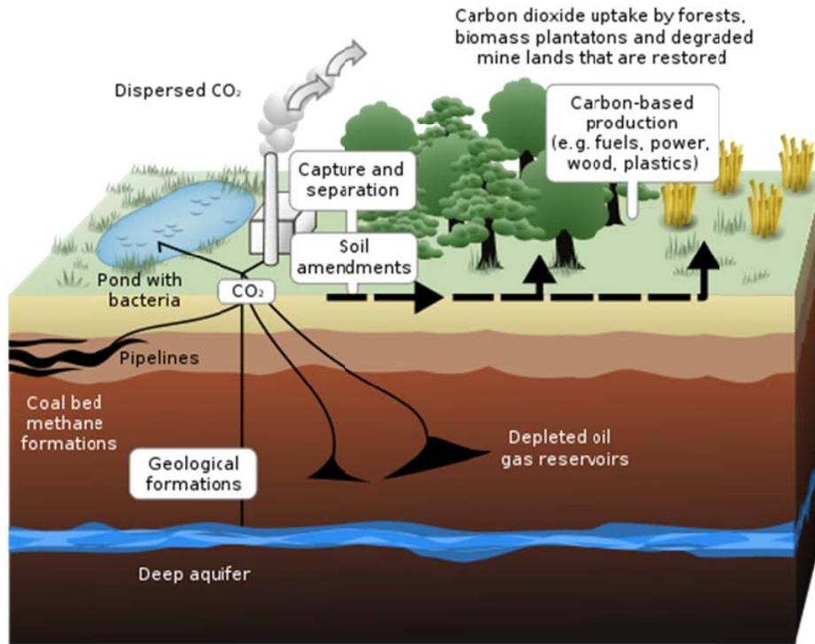
**Fig. (1).** Schematic showing both terrestrial and geological sequestration of carbon dioxide emissions from a coal-fired plant. Rendering by LeJean Hardin and Jamie Payne [3].
