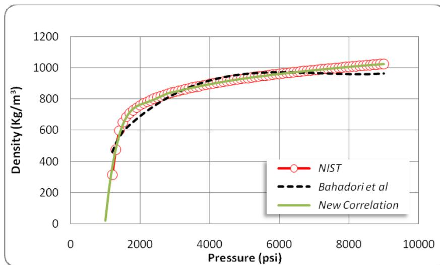
Fig. (4a). Carbon dioxide density changes with pressure at 40°C.
