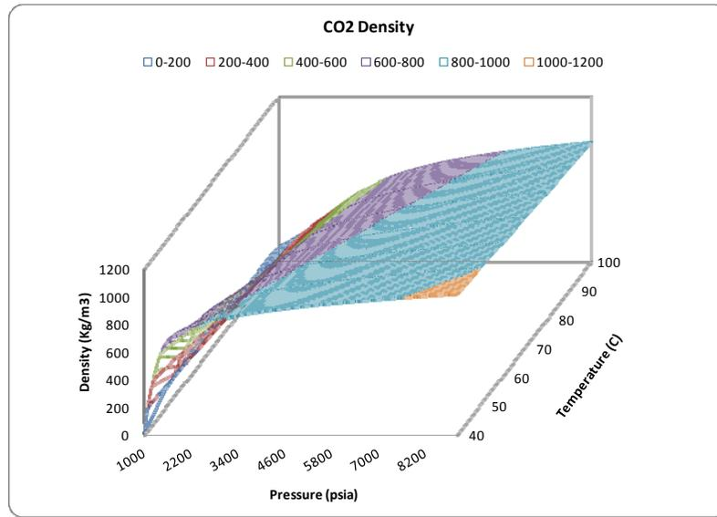
**Fig. (2).** Prediction of carbon dioxide density by Eq. 3 for pressure = 1100 – 9000 psia and temperature = 40 – 100 °C.
