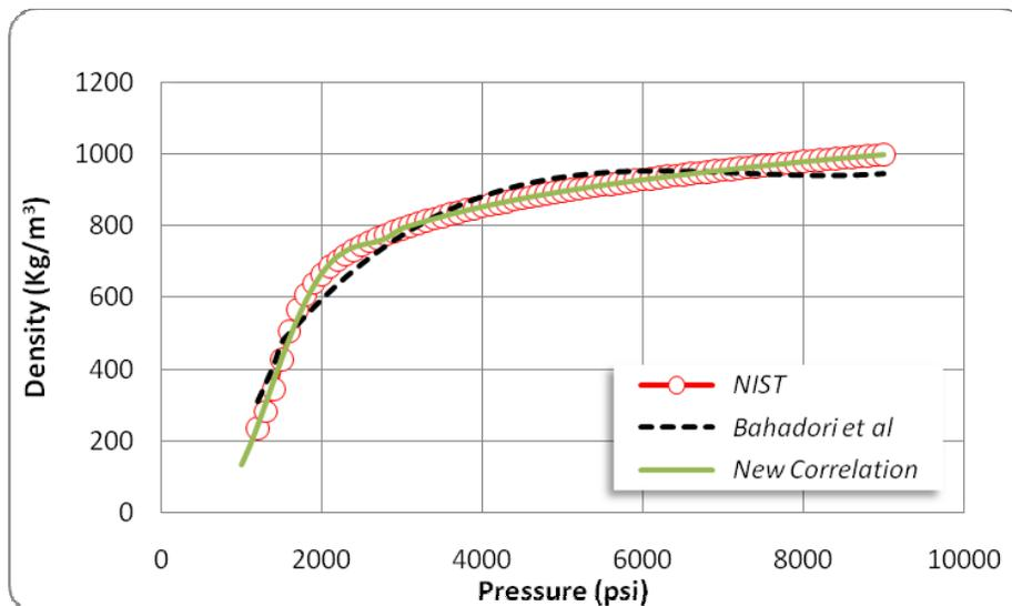
Fig. (4b). Carbon dioxide density changes with pressure at 50°C.
