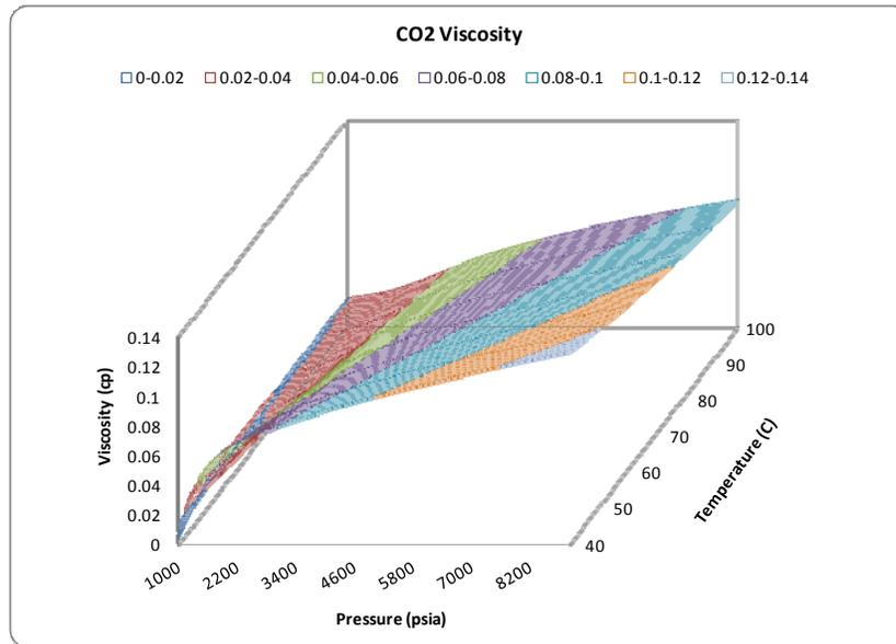
Fig. (3). Prediction of carbon dioxide viscosity by Eq. 5 for pressure = 1100 – 9000 psia and temperature = 40 – 100 °C.
