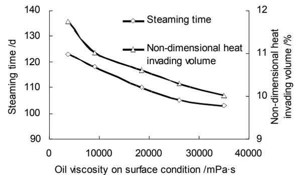
Fig. (4). The influence of oil viscosity on steam breakthrough.
