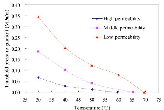
Fig. (5). Threshold pressure gradient vs. temperature of low viscosity of ordinary heavy oil.
