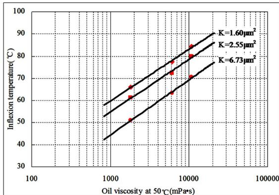
Fig. (8). The fitting curves of inflection temperature and viscosity of heavy oil at 50 °C.
