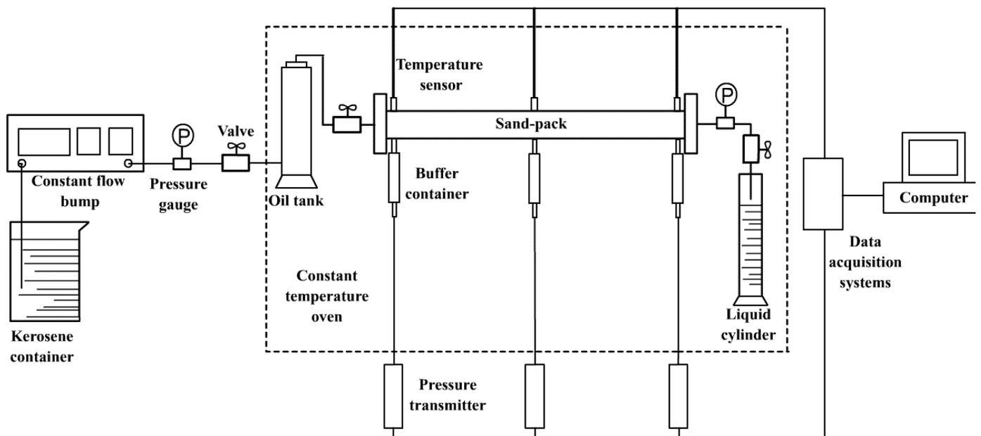
Fig. (1). The Schematic of heavy oil threshold pressure gradient experiment.
