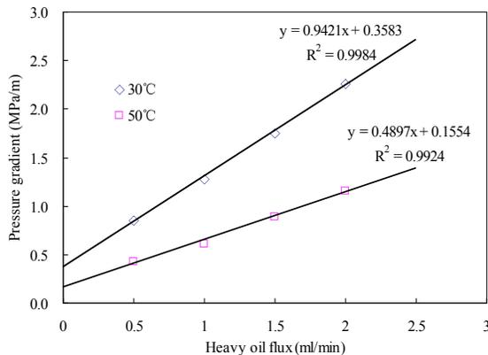
**Fig. (2).** Threshold pressure gradient vs. heavy oil flux at different temperature.
