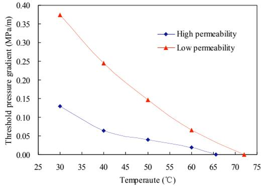
Fig. (6). Threshold pressure gradient vs. temperature of middle viscosity of ordinary heavy oil.
