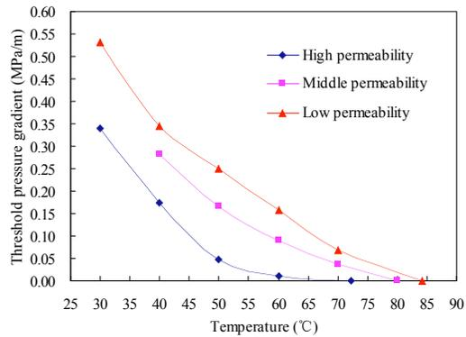
Fig. (7). Threshold pressure gradient vs. temperature of super heavy oil.
