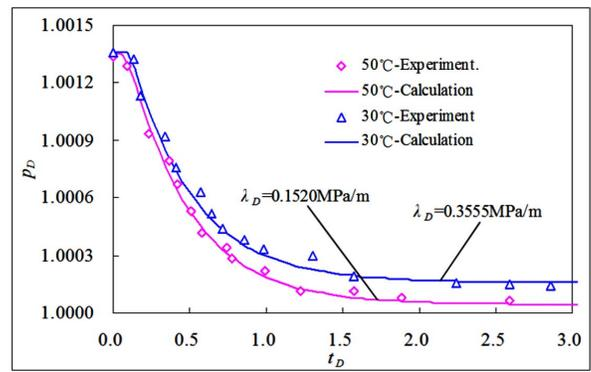
**Fig. (3).** Comparison of dimensionless pressure between experiments and calculations at different temperature.
