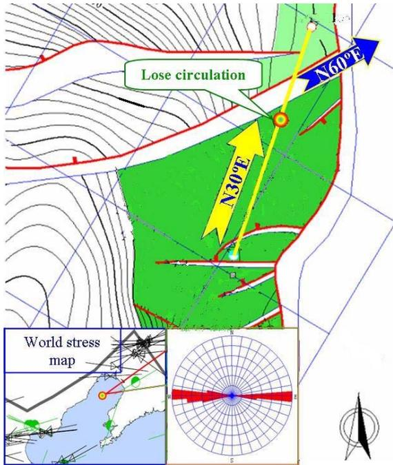
Fig. (5). A directional well in depleted fault-block reservoir in Bohai Bay. ( $\theta=30^\circ, \gamma=20^\circ$ ).
