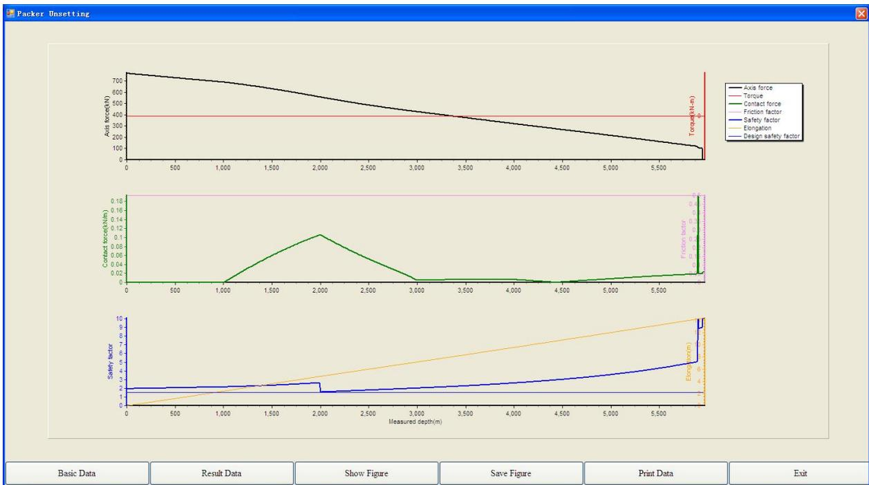
Fig. (5). Mechanical conditions of T-1 well string in packer unsetting.
