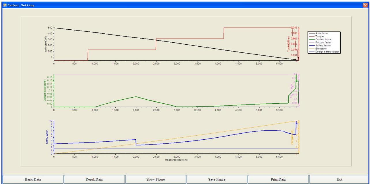
Fig. (3). Mechanical conditions of T-1 well string in packer setting.
