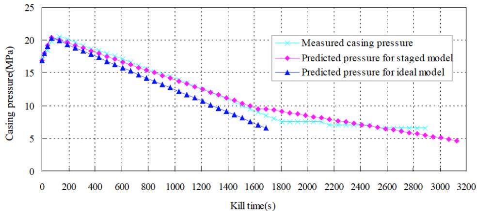
Fig. (3). The comparison of predicted casing pressure and measured pressure.
