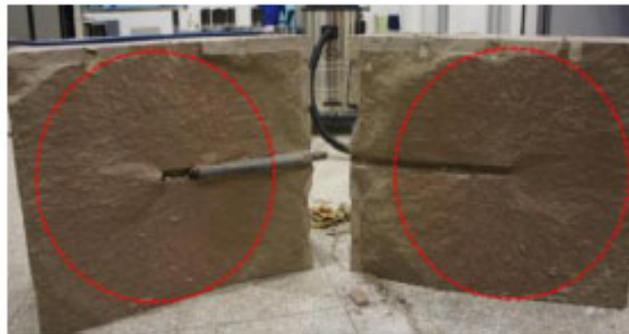
Fig. (5). Hydraulic fracture face after the hydraulic fracturing.
