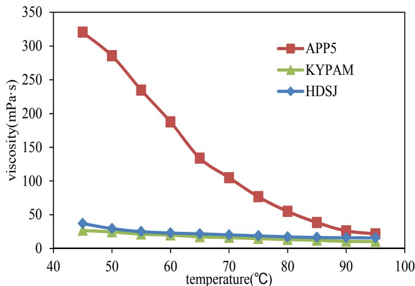
Fig. (2). The relationship between viscosity and temperature.
