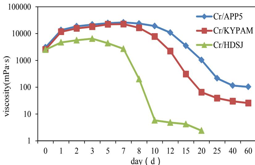
Fig. (3). Plugging agent stability test.
