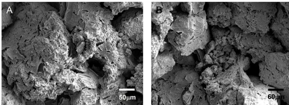
Fig. (8). Corrosion of clay before ASP flooding (A) and after 50 PV ASP flooding (B).
