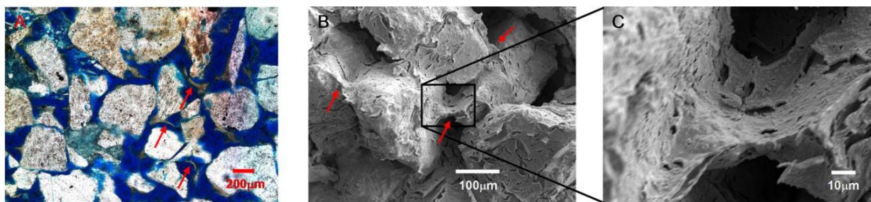
**Fig. (11).** Intergranular character of sandstone after 500 PV ASP flooding. (A): Casting slice image; (B): SEM image; (C): Amplified of middle part of image B.
