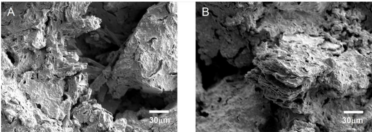
**Fig. (10).** Corrosion of quartz and feldspar before ASP flooding (A) and after 100 PV ASP flooding (B).
