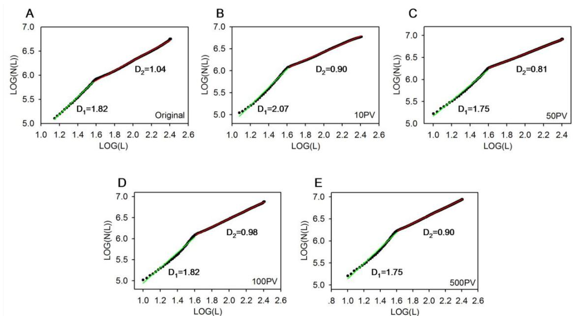
Fig. (5). Graphical plots of logarithms of number of pore with depth L versus logarithms of pore depth. Green and red lines show the linear fit of two scatter spots segments.
