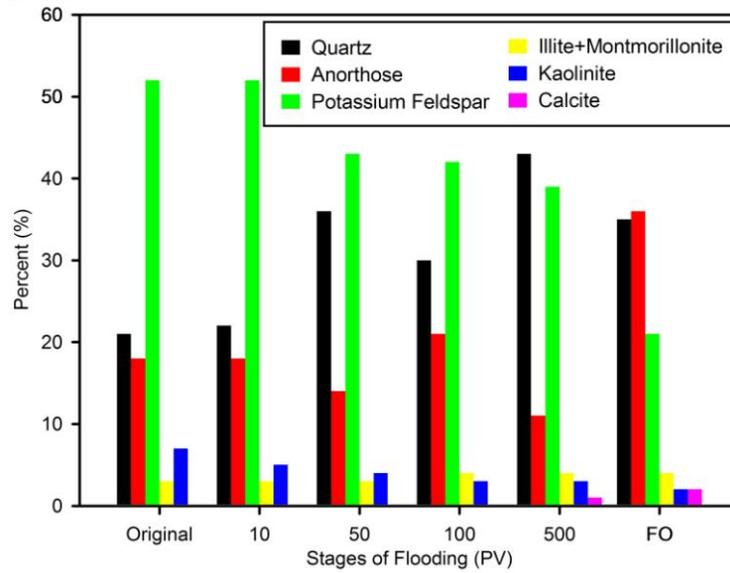
**Fig. (9).** Quality percents of mineral in sandstones at different ASP flooding stages.
