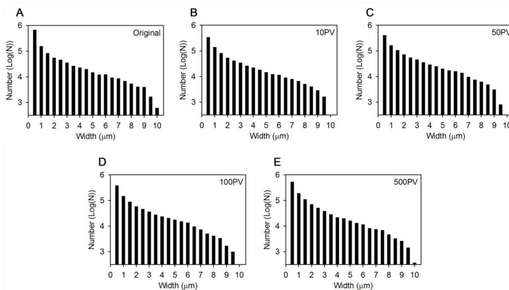
**Fig. (3).** Width distributions of pores at different flooding stages.
