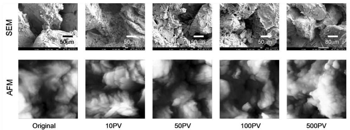
Fig. (2). SEM and AFM micrographs of different flooding stages. The AFM micrographs size is 10 μm × 10 μm. The right gray bar from black to white for AFM images represents the height from 0 μm to 4 μm.
