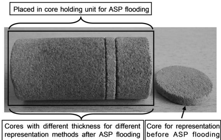
Fig. (1). Cores prepared for laboratory ASP flooding.
