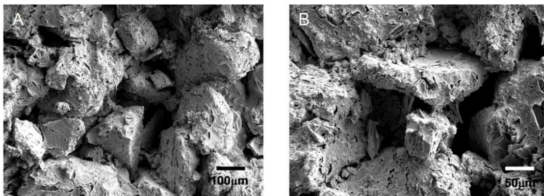
**Fig. (7).** Distribution of intergranular particles before ASP flooding (A) and after 10 PV ASP flooding (B).
