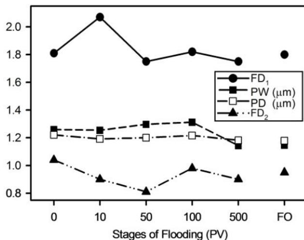
**Fig. (6).** Comparison of mean pore width (PW), mean pore depth (PD), and fractal dimensions (FD1, FD2) at different ASP flooding stages.
