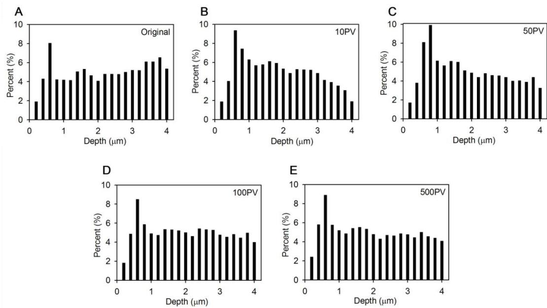
Fig. (4). Depth distributions of pores at different flooding stages.
