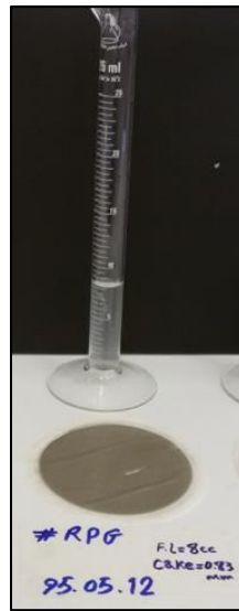
Fig. (3). Amount of filtrate loss and mud cake thickness of Nano DF/RPG.
