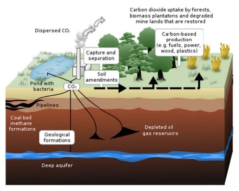
Fig. (1). Schematic showing both terrestrial and geological sequestration of carbon dioxide emissions from a coal-fired plant. Rendering by LeJean Hardin and Jamie Payne [3].
