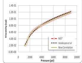
Fig. (5b). Comparison of carbon dioxide viscosity at 50°C as predicted by existing and new correlations.
