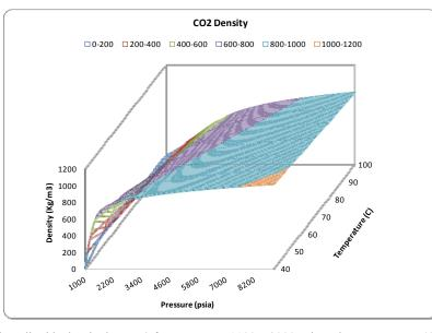
Fig. (2). Prediction of carbon dioxide density by Eq. 3 for pressure = 1100 - 9000 psia and temperature = 40 - 100 °C.
