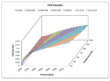
Fig. (3). Prediction of carbon dioxide viscosity by Eq. 5 for pressure = 1100 - 9000 psia and temperature = 40 - 100 °C.
