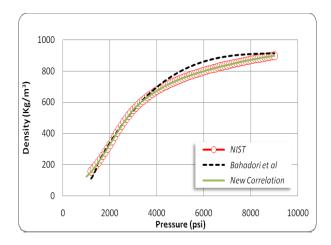
Fig. (4f). Carbon dioxide density changes with pressure at 90°C.
