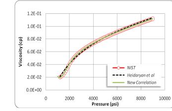
Fig. (5c). Comparison of carbon dioxide viscosity at 60°C as predicted by existing and new correlations.
