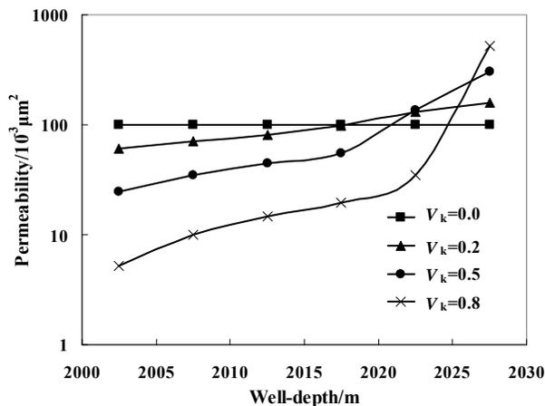
Fig. (1). Permeability distribution along the well bore.
